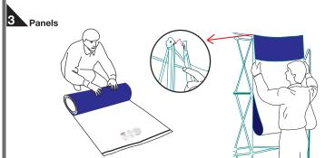
Panels attach with magnets and align down centre of magnetic bars
