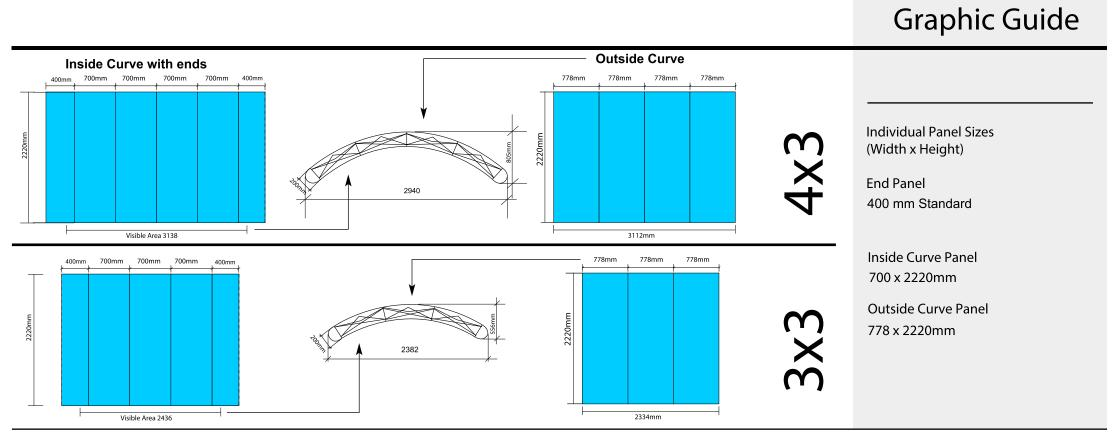
A Stand is described by the number of frame squares wide (panels) x the number of frame squares high. Panel height is 2220mm. Stand height is 2240mm.
