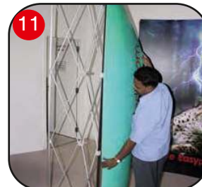
10-12. Hook graphic panel onto hookstuds and attach edge of panel to align with centre of magbar (on both edges of graphic panel). Attach remaining two panels similarly.
